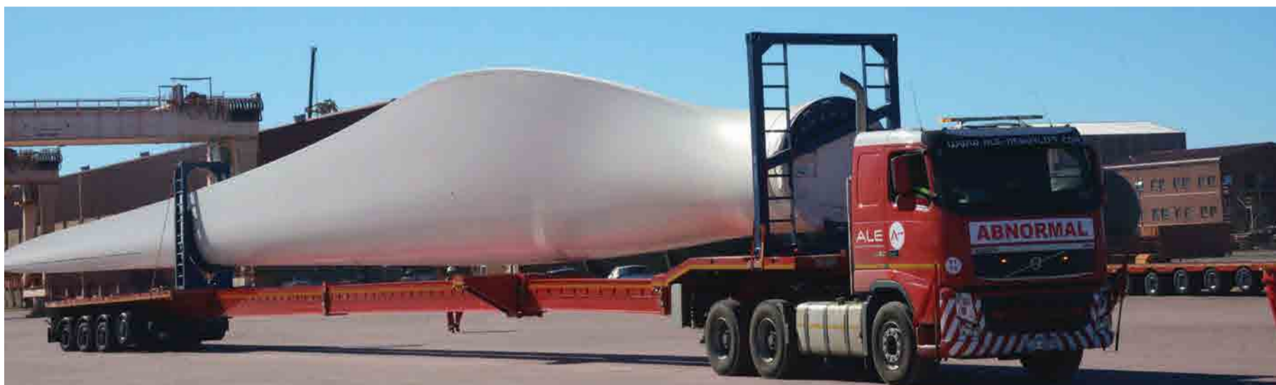
Each blade had to be transported individually. The wind farm has 66 turbines each with three blades, so that made for almost 200 trips. Photo: Supplied by Cookhouse Wind Farm
