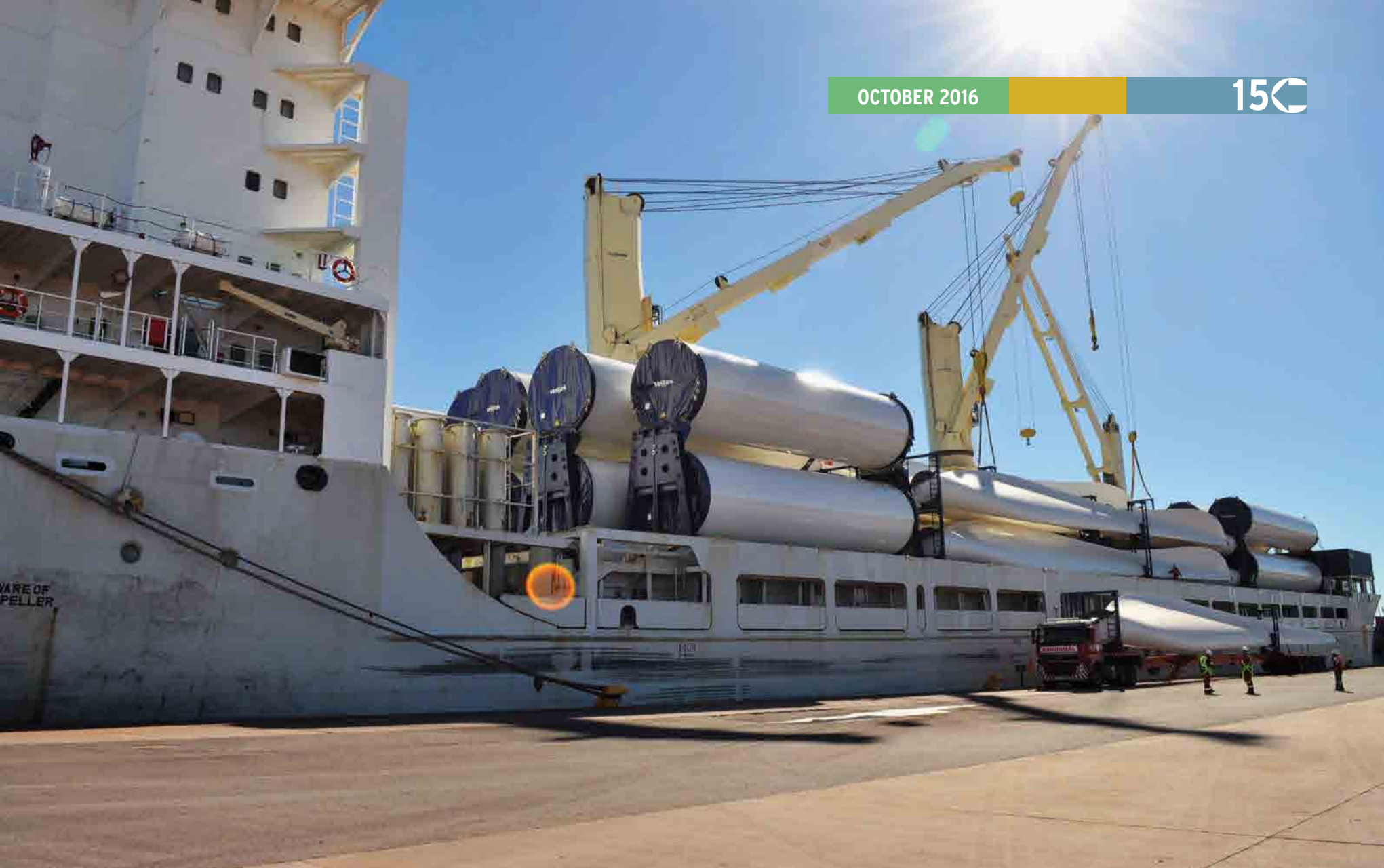
Before construction the turbine towers and blades arrived after being manufactured in India. Photo: Supplied by Cookhouse Wind Farm
